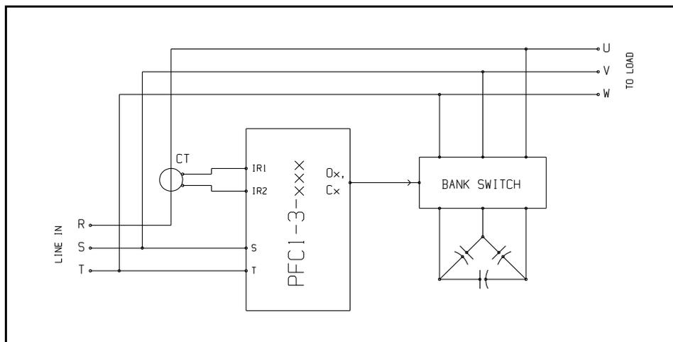
Typical three-phase power factor correction PFC1 system. Only one capacitor bank is shown for clarity. The bank switch can either be a set of solid state switches or a relay contactor.
