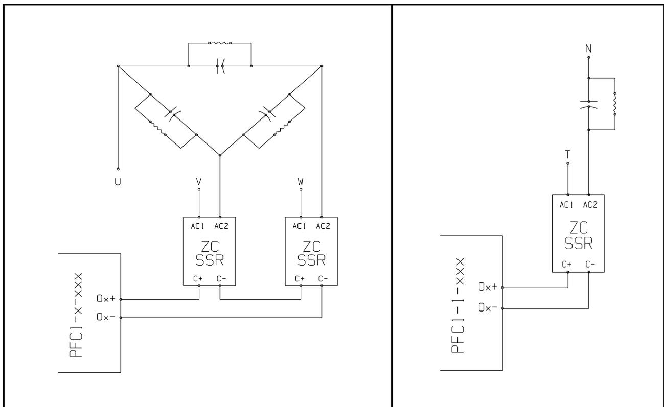
Typical solid state relay bank switch connection in three-phase (left) and single-phase (right) line systems. The SSRs must be of the zero-crossing (or line synchronized) type to ensure that the capacitors are switched in when the line voltage equals the capacitor voltage thus eliminating capacitor inrush current and extending capacitor service life. The capacitor discharging resistors are for safety only and can be any suitable value giving minimum heat dissipation while connected to the line.
