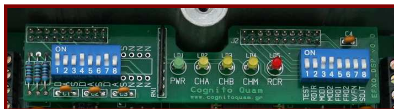
Detail showing the function DIP switches and status LEDs.
